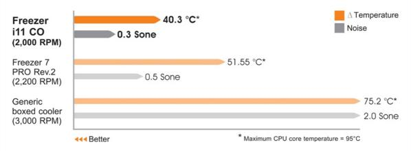
Cooling Performance & Noise Level on Intel Core i7 4930K (Full Load)
